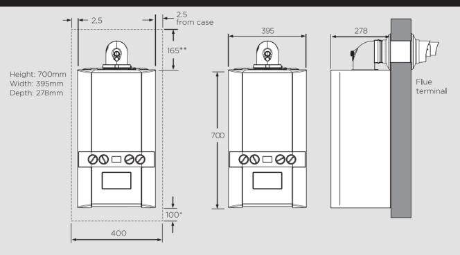
**Note:** The minimum front clearance when built in to a cupboard is 5mm from the cupboard door but 450mm overall clearance with the cupboard door open is required for servicing. \*Bottom clearance after installation can be reduced to 5mm. However, 100mm is required for servicing.
